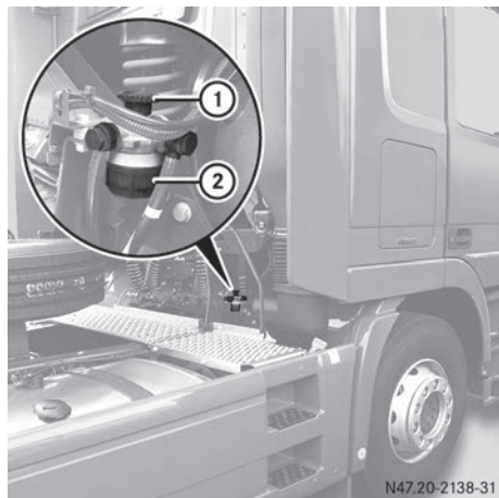
Example: hand pump on the rear wall
