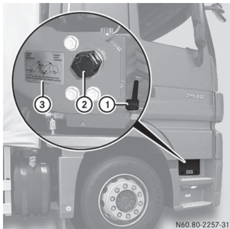
Example: tilting pump, in doorway on the right-hand side, behind the flap
