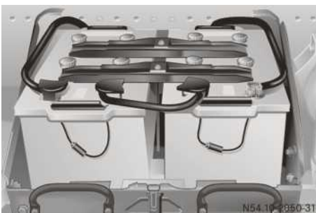
Example: battery carrier on the side of the chassis
