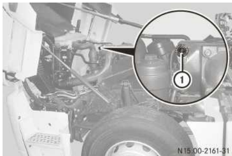
External engine start/engine stop switch mounted on the engine (example: engine from 260 kW)
