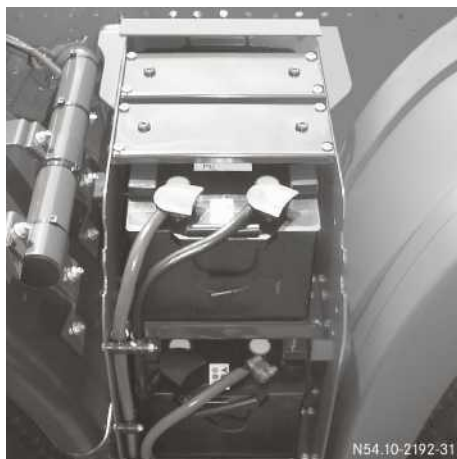
Example: battery support frame on the side of the chassis – batteries arranged one above the other
